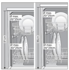
If required, the height of the top basket can be adjusted in order to create more space for large utensils either in the top or bottom basket.
